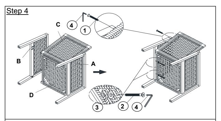
Attach Right Leg (B) to Seat Panel (D) by using Bolts(2), Flat Washer (3) with Allen Key (4).
