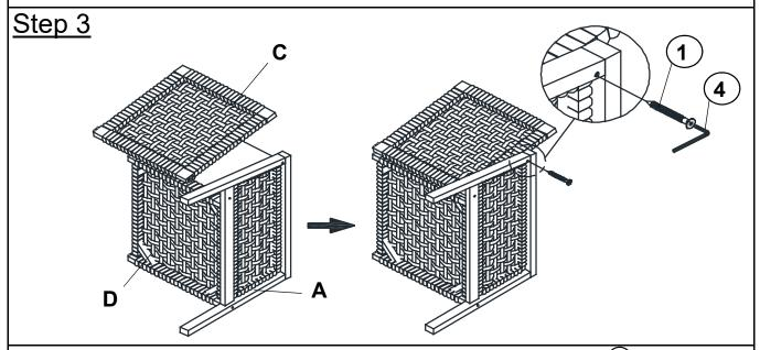
Attach the Back Panel (C) to the Left Leg (A) by using Screw (1) with Allen Key (4).
