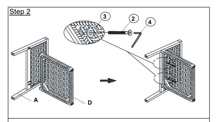
Position the Seat Panel (D) to the Left Leg (A) as shown in the above picture. Attach the Seat Panel (D) to the Left Leg (A) by using Bolts(2), Flat Washers (3) with Allen Key (4).
