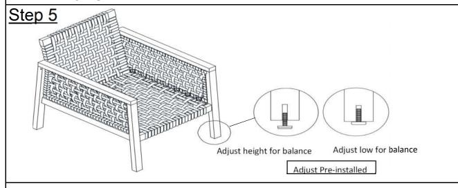
With the assistance from your adult partner, stand the Chair up Inspect the Chair and make sure all parts are adequately connected. Carefully sit onto the Chair. This pressure will help align all parts at all joints.
