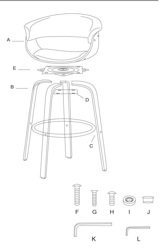
Attach Connector (D) to four pieces of Leg (B) by using Long Semicircle Head STEP 1 Bolt (F) and Big Allen Key (K) as shown in below diagram, please do tighten bolts 70%.
