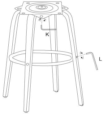
STEP 5 Attach Swivel Mech (E) to the Seat (A) by using Long Semicircle Head Bolt (F), Washer (I) and Big Allen Key (K) from the front side, by using Short Semicircle Bolt (H) and Big Allen Key (K) from the back side as shown in below diagram. Please make sure to tighten bolts (G) and bolts (H) 100% in this step.
