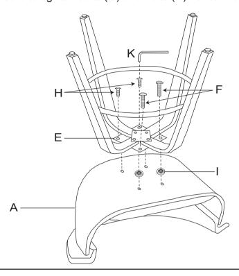
Use your body weight to adjust balance of this counter stool, then recheck and STEP 6 ensure 100% tighten all the bolts all the way.
