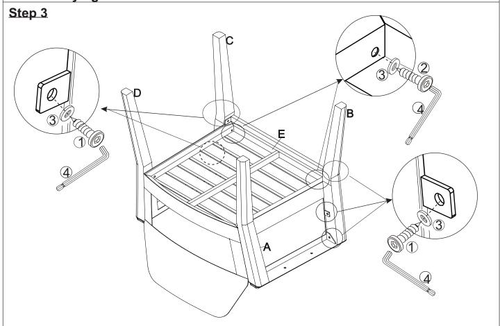
Attach the Front Right Leg (B) and Front Left Leg (C) to the Seat Frame (E) using Screws (1), Screws (2), Washer (3) and Allen Wrench (4). **Do not fully tighten the Screws**.
