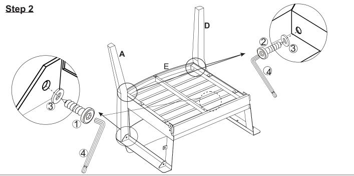
Place the Seat Frame (E) facedown on a clean, non-marring surface as shown in above picture. Attach the Back Right Leg (A) and Back Left Leg (D) to the Seat Frame (E) by using Screw (1), Screws (2), Washers (3) and Allen Wrench (4). **Do not fully tighten the Screws.**
