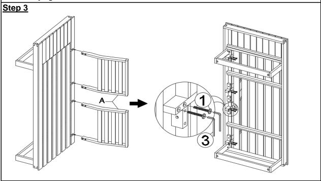
With the help of your adult partner, stand the assemble in step 2 up, then attach the first Backrest Panel (A) to the assemble using Bolts (1) and the Allen Key (3).
