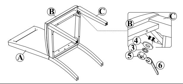
Step 3: Place the Chair to upright position on flat surface and adjust legs until level and does not wobble Fully tighten all bolts and hex nuts with Wrench (6). Assembly of product is completed.
