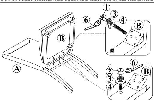
Step 1: Place the Chair Back (A) on the floor. Attach Seat Box w/Seat Cushion (B) to the Chair Back (A) by inserting the Short Bolt (2), Lock Washer (3), Flat Washer (4) into the holes at the rear bar of the seat frame. Attach Long Bolt (1), Lock Washer (3), Flat Washer (4) into the holes at the rear corner block of the seat box. Tighten all Bolts with Wrench (6). Do not fully tighten.
