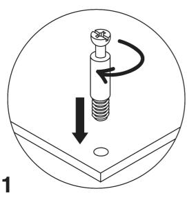
Screw the cam bolt into panel.
