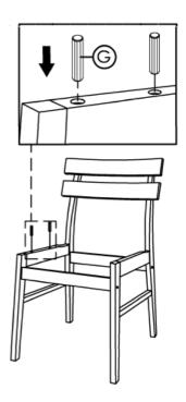
Insert Wood Dowel (G) into the designated hole on Right Frame as shown.
