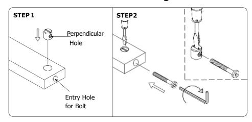
Insert Barrel Nut with the perpendicular hole facing and in-line with the drill hole that the bolt is to be inserted.
