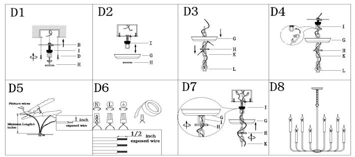
Step D1: .Attach single bar (B) to outlet box with mounting screw (D). The side of single bar marked "GND" must face out Unscrew threaded ring (H) from collar loop (I)
