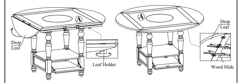
Step 3: Turn the table to upright position (\*Note: It is recommended to use two or more person to turning the table). Twisting the Leaf Holder to release the Drop Leaf of the Table Top (A), folding up the Drop Leaf and pull the Wood Slides to keep the Drop Leaf is opened, as the picture shown.
