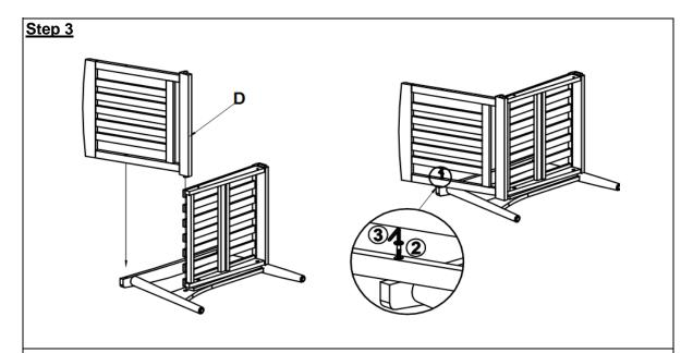
Position the Backrest Panel(D) to the Seat Panel(C) and the Right Leg Panel(A) as shown in the above picture.
