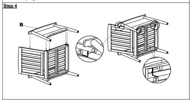
Position the Left Leg Panel(B) to the Seat Panel(C) and the Backrest Panel(D) as shown in the above picture.
