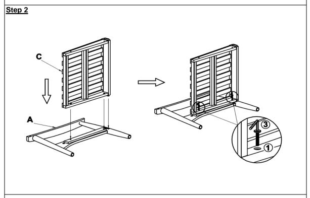
Position the Seat Panel(C) and the Right Leg Panel(A) as shown in the above picture. Then secure the Seat Panel(C) to the Right Leg Panel(A) using 2 Bolts( $\widehat{\ \ }$ ) and the Allen Key( $\widehat{\ \ \ }$ ).
