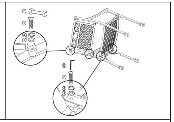
Repeat the same step to attach Backrest Panel(A) and Seat Panel(B) to Right Arm Leg with Pre-attached Levellers(D). **DO NOT fully tighten at this stage.**
