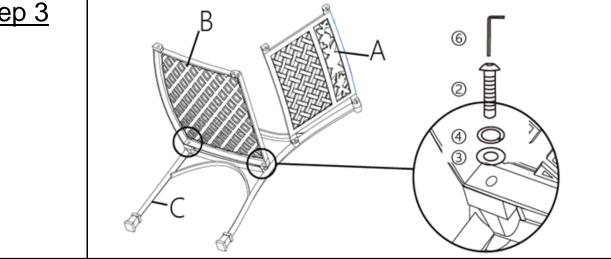
Then attach Chair Seat Panel(B) to Left Arm Leg with Pre-attached Levellers(C) using Bolts(2), Spring Washers(4) and Washers(3) with Allen Wrench(6).
