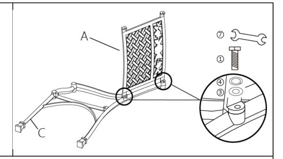
Attach Backrest Panel(A) to the Left Arm Leg with Pre-attached Levellers(C) using Bolts(1), Spring Washers(4) and Washers(3) with Spanner(7).
