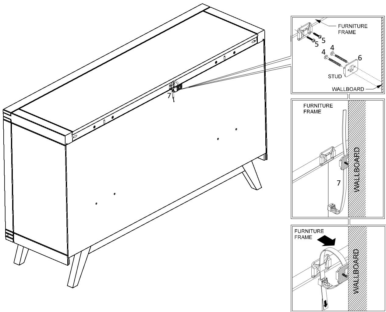
**STEP (A)** Locate a wall stud behind your furniture. Position a bracket on the stud approximately 1" below the top of the furniture. Mark & drill pilot hole into the center of the stud with a 3/32" drill bit. Attach the bracket to the stud with the screws provided (B).
