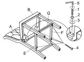
1. Loosely attach the Linen Fabric Seat(B) to the Stool Back(A), using Bolts(5+1+2+3) to tighten, as shown.
