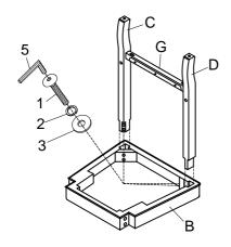
1.Loosely attach the left leg(C) and Right Leg(D) to the Linen Fabric Seat(B), using Bolts(5+1+2+3) to tighten, as shown.
