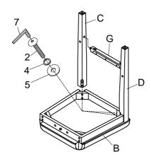
1.Loosely attach the left leg(C) and Right leg(D) to the Linen Fabric Seat(B), using Bolts(7+2+4+5) to tighten, as shown.
