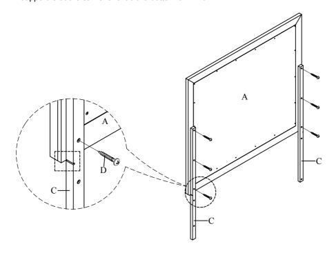
Place the mirror with support on the top of Dresser (B). Then align center as shown and using PH Screw (D). Tighten using Phillips Screwdriver (not provided).
