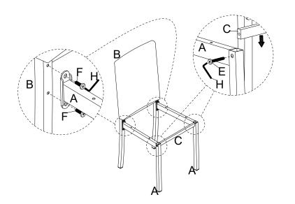
Take the Allen Key, and turn the bolts until the legs are secure. DO NOT TIGHTEN COMPLETELY. Stop when you feel you are adding force to tighten the bolts.
