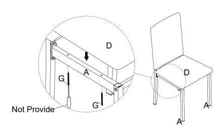
Stand chair up on an even surface and check that it is balanced. If there is a slight wobble, apply downward pressure in the corner where a leg is uneven. Keeping pressure in that corner, tighten all bolts. If balanced, apply downward pressure evenly in the center and tighten all bolts. Do not over-tighten beyond hole depth.
