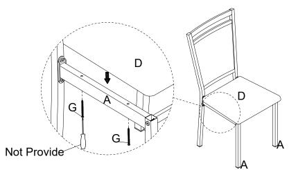
Stand chair up on an even surface and check that it is balanced. If there is a slight wobble, apply downward pressure in the corner where a leg is uneven. Keeping pressure in that corner, tighten all bolts. If balanced, apply downward pressure evenly in the center and tighten all bolts. Do not over-tighten beyond hole depth.
