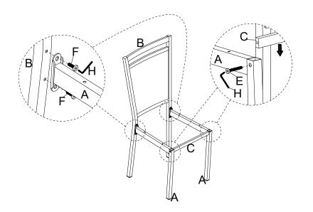
Take the Allen Key, and turn the bolts until the legs are secure. DO NOT TIGHTEN COMPLETELY. Stop when you feel you are adding force to tighten the bolts.
