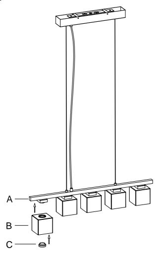
Firstly, remove the Bolt (H) from the Ceiling Base of Light Body (A), take out the bracket and assemble it to the ceiling using Bolt (E) & Flat Washer (D) by screwdriver. Then connect the Wire Connector (F) and Wire Connector (G) together with cable. Finally, put the ceiling base back to cover the bracket and using Bolt (H) by screwdriver to fix them.
