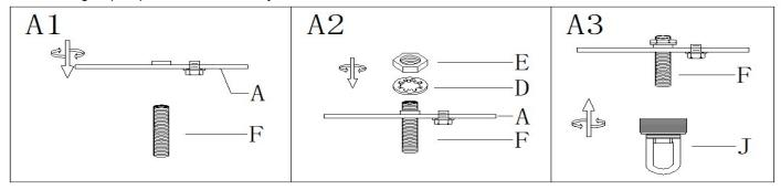
Step A1: Thread the single bar(A) onto the nipple (F), At this point need note that: the side of single bar marked "GND" must face to the down.
