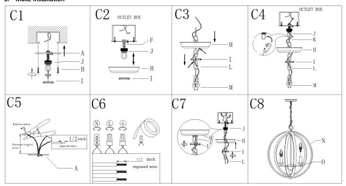
Step C1: Remove the threaded ring (I) from collar loop(J).
