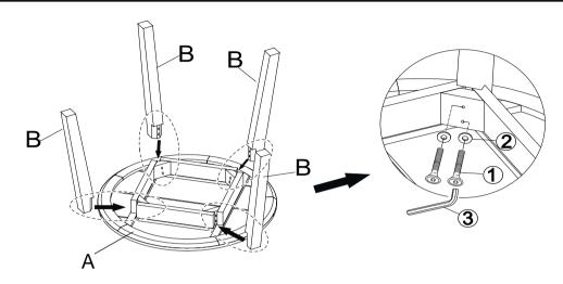
Place the Table Top (A) with its underside facing upwards onto a clean, soft surface to avoid any scratch or damage to the product.
