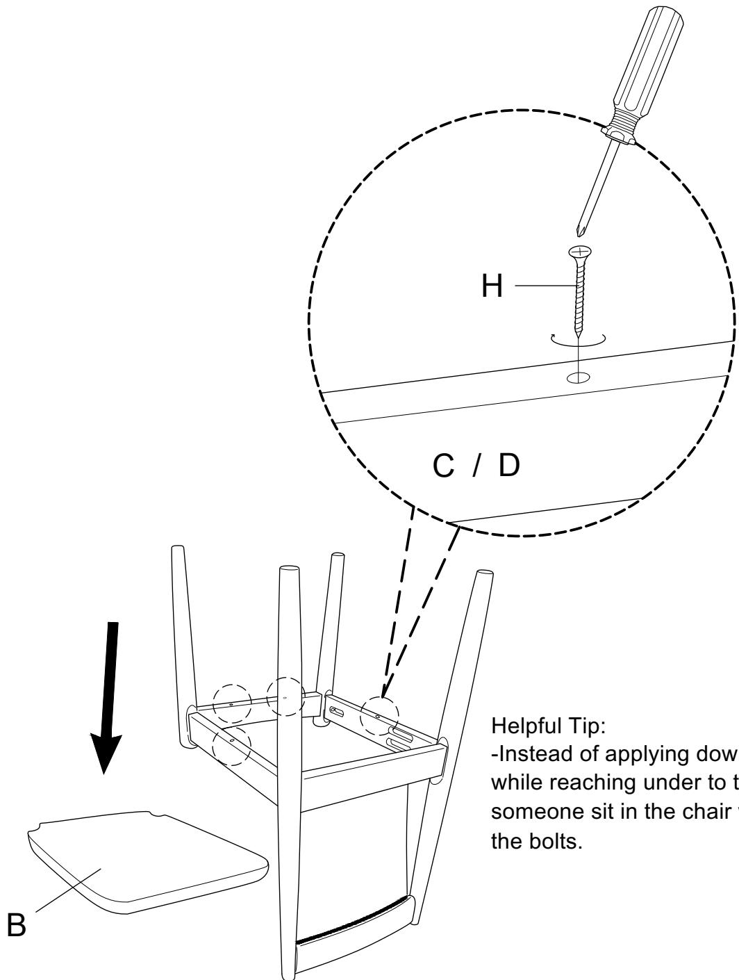
Stand the chair up on even surface and check that it is balanced. If there is a slight wobble, apply downward pressure in the corner where a leg is uneven. Keeping pressure in that corner, tighten all bolts. If balanced, apply downward pressure evenly in the center and tighten all bolts. Do not over-tighten beyond hole depth.
