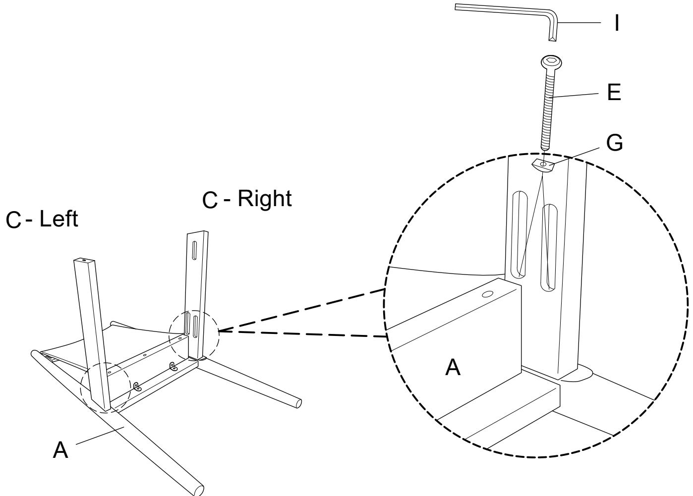
Take the Allen Wrench, and turn the bolts until the legs are secured.
