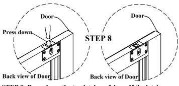
STEP 8: Press down the top latches of door. If the latches are at lower possition already, please go to Step 9.
