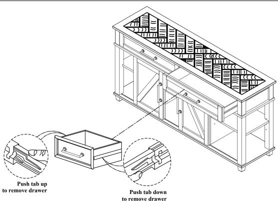
To remove drwer, simmultaneously pull tab up on one side and push down on the other and remove drawer
