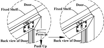
STEP 9: Use your forefingers to press in the buttons at the side of the Latches so that the Latches go up into the U-Track.
