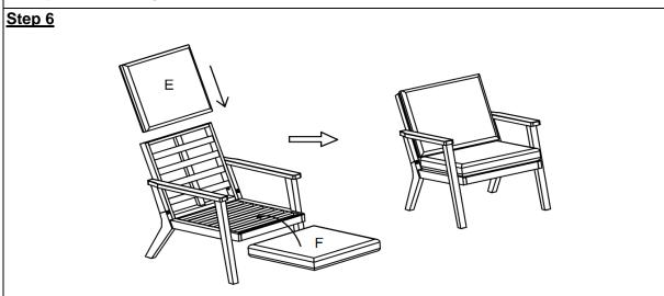
Place the Back Cushion(E) and the Seat Cushion(F) onto the Backrest(D) and the Seat Panel(C) as shown in the above picture.
