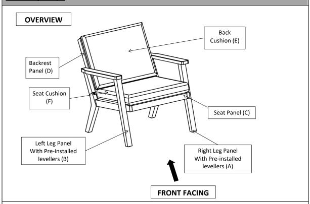
This Chair has multiple parts and may require up to some 30 minutes to assemble. To give you an overview of the Chair, the above picture is to help you put the various parts into perspective. Please read through the instructions here below to familiarise yourself with the parts and steps before assembly.
