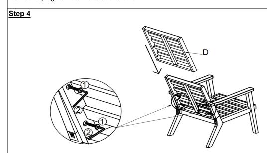
Place the Backrest Panel(D) into the Seat Panel(C) as shown in the above picture. Then secure the Backrest Panel(D) to the Right Leg Panel With Pre-installed Levellers(A) using 2 Bolts(1) and the Allen Key(2).
