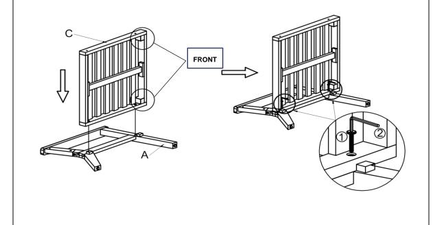
Position the Seat Panel(C) to the Right Leg Panel With Pre-installed Levellers(A) as shown in the above picture.
