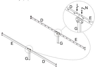
Attach Front & Rear Rail Section (D & E) to Headboard (A), Footboard (B) and Headboard Leg (C) using Bolt (K) with Allen Key (N).
