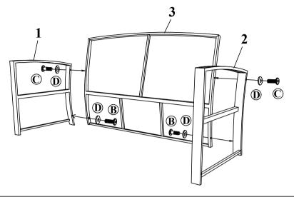
Step 1 Connect Bench Left Frame (1) & Bench Back Frame (3) & Bench Right Frame (2) & tighten Bolt (B),(C) with Allen key (E)
