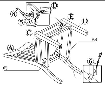
Step 2: Attach the LSF/RSF Fron Leg (C/D) to Seat Box w/Wood Seat (B) by using Flat Washer (4). Lock Washer (3) and Hex Nut (5) secure by Open Wrench (8). Attach the Front/LSF/RSF Stretcher (E/F/G) to LSF/RSF Front Leg (C/D) and Chair Back (A) by securing the Screw (6) with Phillips-head screw drivers (Not provided).
