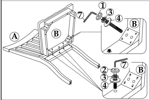
Step 1: Place the Chair Back (A) on the floor. Attach Seat Box w/Wood Seat (B) to Chair Back (A) by using the Flat Washer (4), Lock Washer (3), Long Bolt (1) into the holes at the rear corner block of the seat box. Insert Flat Washer (4), Lock Washer (3) and Short Bolt (2) into the holes at the rear of the seat frame.
