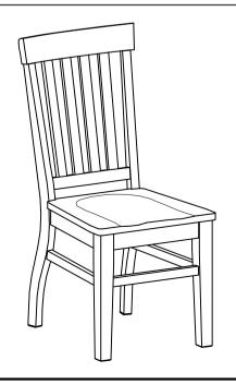
Step 3: Place the side chair to upright position on flat surface and adjust chair legs until level and chair does not wobble. Fully tighten all Bolts and Hex Nuts at this time. Assembly product is completed.
