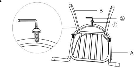
Place the Back(A) facedown onto a clean, non-marring surface. Align the Back(A) to Chair Legs(B) as shown above.
