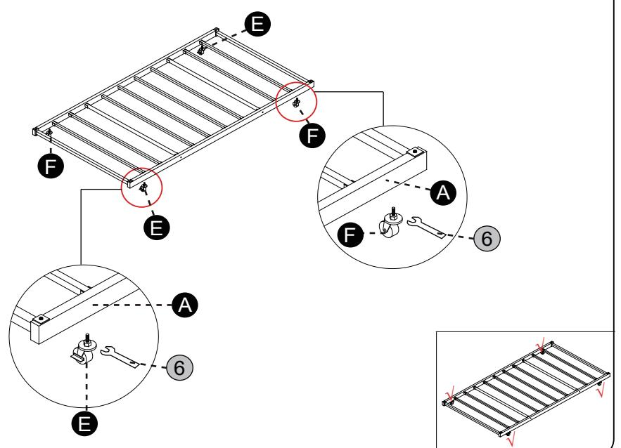
5 Check and tighten all screws
