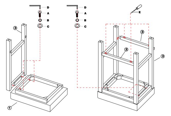
NOTE: DO NOT TIGHTEN ALL THE BOLTS UNTIL THEY ARE INSTALLED IN CORRESPONDING HOLES!
