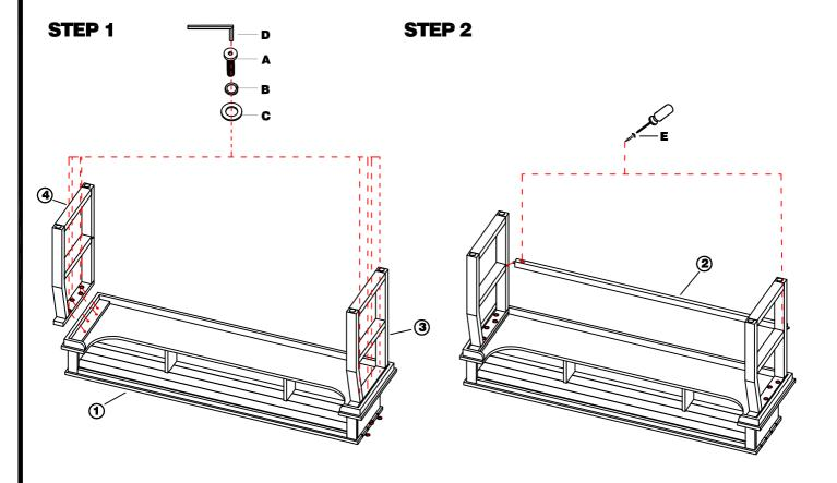
NOTE: DO NOT TIGHTEN ALL THE BOLTS UNTIL THEY ARE INSTALLED IN CORRESPONDING HOLES!
