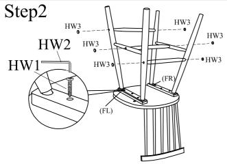
Position the frame assembly into the bottom of chair seat. Align and tighten bolt chair seat and frame using the Screw (HW1) with Allen Wrench (HW2). Tighten all the screw in Step 1 and Step 2
