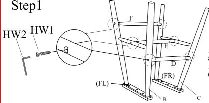
Assemble Short stretcher (D), Middle stretcher (E), and Long stretcher (F) using Screw (HW1) and Allen Wrench(HW2). (Do not tighten yet.)
