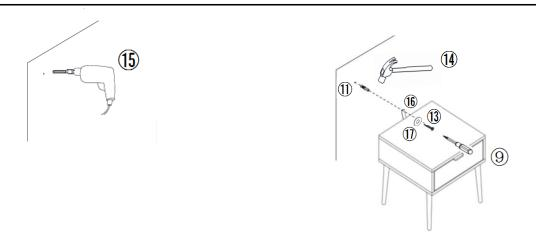
Drill one mounting position on the wall with Power Drill(15), insert Wall Anchor(11) into drilled mounting position on the wall with Hammer(14), Move the cabinet back to the wall, lock by Screw(13) and Metal Gasket(17) with Screwdriver(9).
