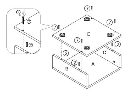
Insert Dowel(②) into Left Side Panel(B) and Right Side Panel(C), attach Bottom Panel(E) to the Dowel on Left Side Panel(B) and Right Side Panel(C) using Screw(⑦) with Screwdriver(⑨).
