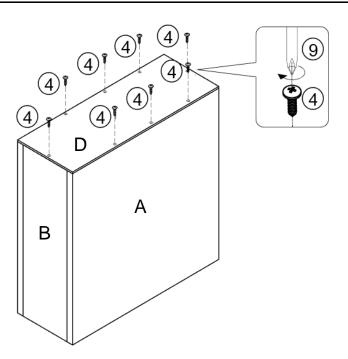
Attach Back Panel(D) to the Top Panel(A), Left Side Panel(B), Right Side Panel(C) and Bottom Panel(E) using Screw(4) with Screwdriver(9) as shown.
