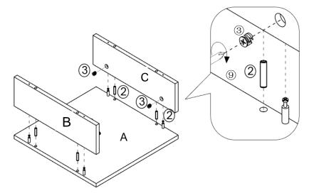
Insert Dowel(②) into the mounting positions on Left Side Panel(B), Right Side Panel(C) and Top Panel(A), Insert Cam Nut(③) into the mounting positions on Left Side Panel(B) and Right Side Panel(C), lock by turning Cam Nut(③) with Screwdriver(⑨)
