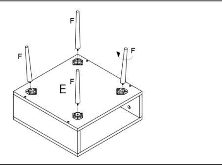
Attach Leg(F) to the Bottom Panel(E), and then turn all legs clockwise to fasten them tightly.
