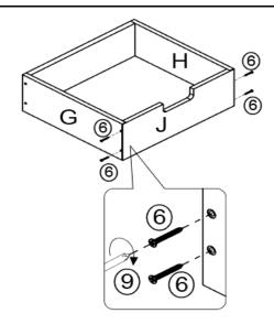
Attach Drawer Front Panel(J) into the Drawer Left Side Panel(G) and Drawer Right Side Panel(H) using Screw(6) with Screwdriver(9) as shown.
