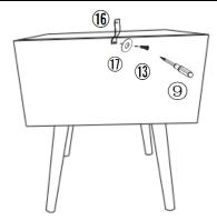
Attach Restraint Strap(16) to the Upper Back Bar(H) using Screw(12) and Metal Gasket(17) with Screwdriver(9).
