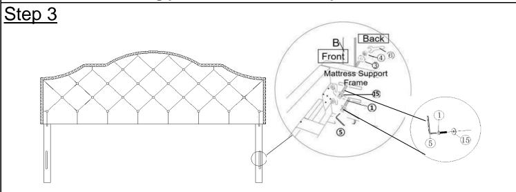
With the assistance of your adult partners, turn over the assembled rails. Attach Support Leg(B/C) to the assembled Rail using Blots(1), Washers(3), Washers(15) and Nuts(4) with Allen Key(5) and Wrench(6).
