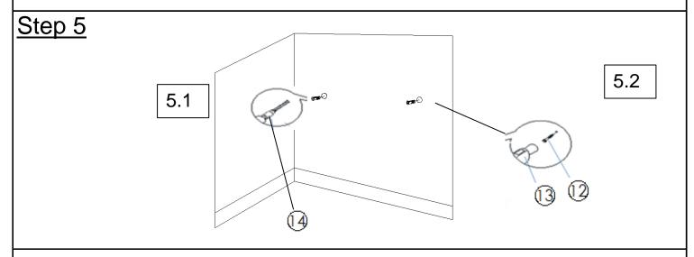
5.1) Drill two holes on wall at the same height as Metal Pad(110) on Headboard with Power Drill(114).
