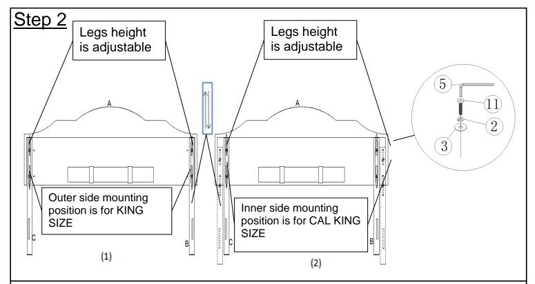
Align the mounting positions on Headboard(A) to those on Left Support Leg(B).
