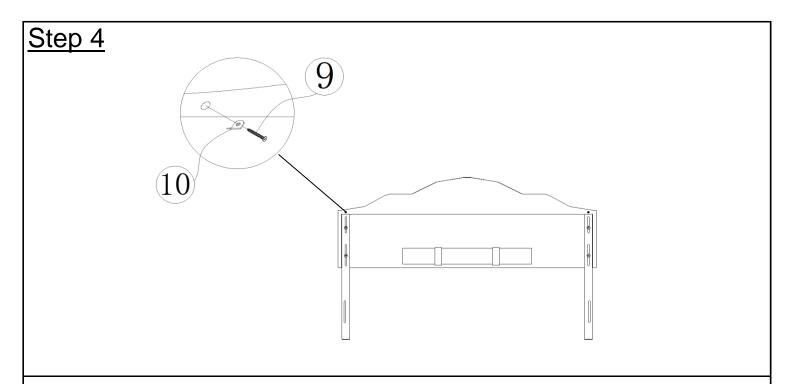
Firstly, turn back the Headboard. Locate the two marks on the product. Then, attach Metal Pads(10) to the back of Headboard(A) using Screws(9). Make sure two parts are connected and securely locked into headboard.
