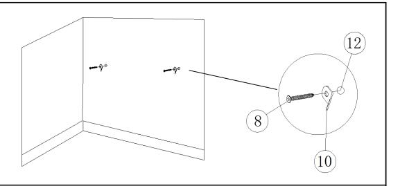
Put the Headboard against the wall where desired and mark the location for the Metal Pads(1) to be the same height as the top of the Headboard. Attach Metal Pads(1) to Wall Plugs(1) using Screws(8). Note: The Metal Pads need to be secured to solid, load bearing surface.
