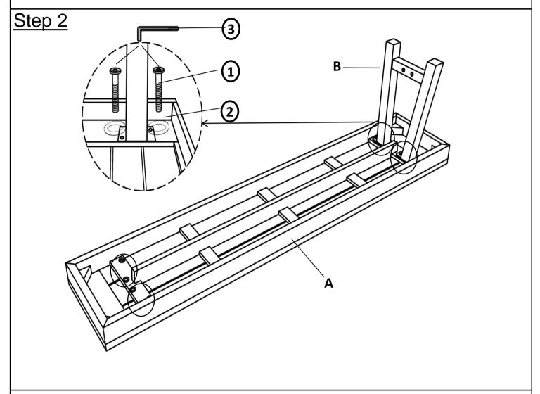
Place the Seat Panel(A) facedown onto a clean, non-marring surface. Attach Iron Legs(B) to Seat Panel(A) using Bolts( $\widehat{1}$ ) and Washers( $\widehat{2}$ ) with Allen Key( $\widehat{3}$ ).
