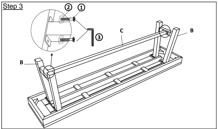
Attach Support Bar(C) to Iron Legs(B) using Bolts(1), and Washers(2) with Allen Key(3) as pictured above.
