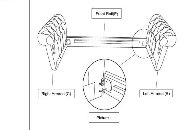
With the assistance of your partner,slide the hook in the eng of Front Rail(E) into the bolts on the Left Armrest(B) and Right Armrest(C), as shown in Picture 1.
