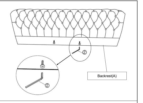
Loosen the 2 bolts in Backrest(A) around half inch by Allen Key( $\mathfrak{D}$ ).
