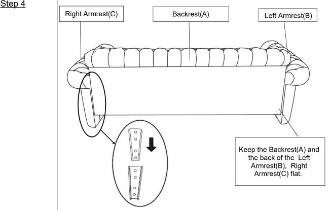
Slide the Tapered Connectors on the Backrest(A) into the Tapered Connectors on the Left Armrest(B) as shown in the picture.
