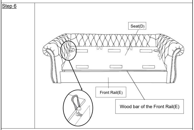
With the assistance of your partner, lift the rope on the two sides of Seat(D) by hand. Put the Seat(D) on the wood bar of the Front Rail(E) and then slowly place it down as shown above. **Note:All the u-shaped iron sheet need clamped to the bolt.**
