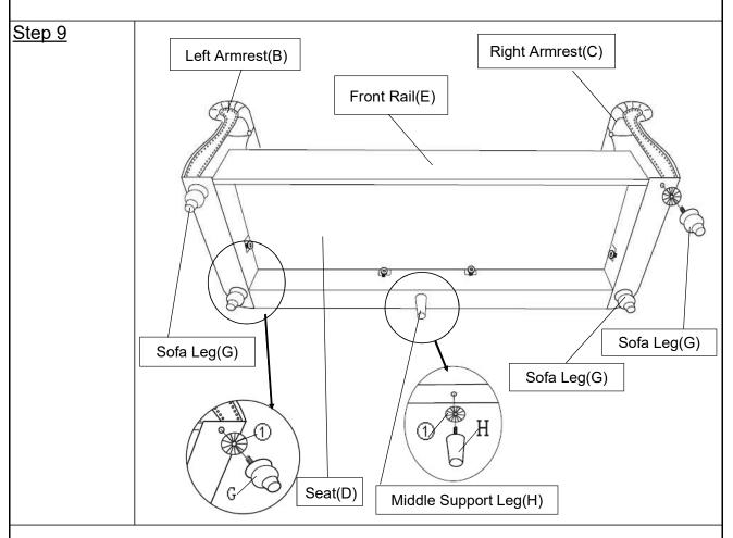
Install the Leg(G) at the bottom of Left Armrest (B) and Right Armrest(C) by placing Plastic Washer( $\bigcirc$ ) on the threaded stem.
