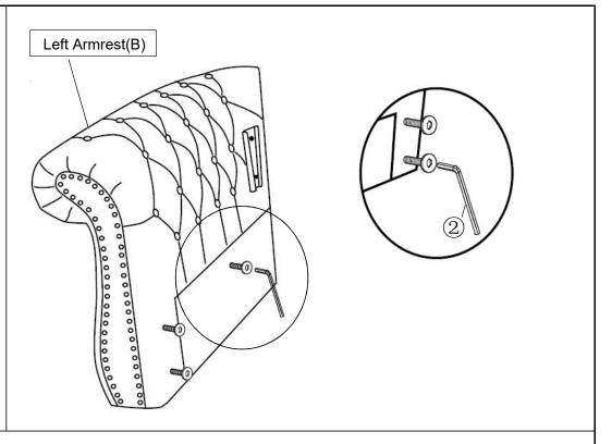
Open the carton and place all the parts on a clean, non-marring surface. Loosen the 3 bolts in Left Armrest(B) around half inch by Allen Key(②). Repeat the same step to loosen 3 bolts in Right Armrest©.
