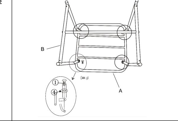
Attach Table Leg (B) to Table Top (A) with Bolts(1) and Washers (4) using the Allen Key (3).
