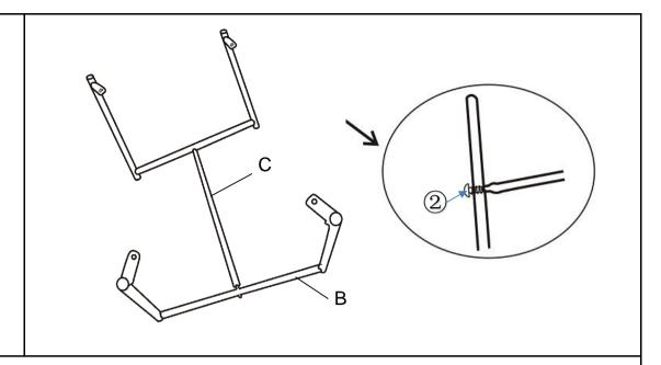
Attach the Support Rod (C) to Table Leg (B) with Bolts(2) using the Allen Key (3).
