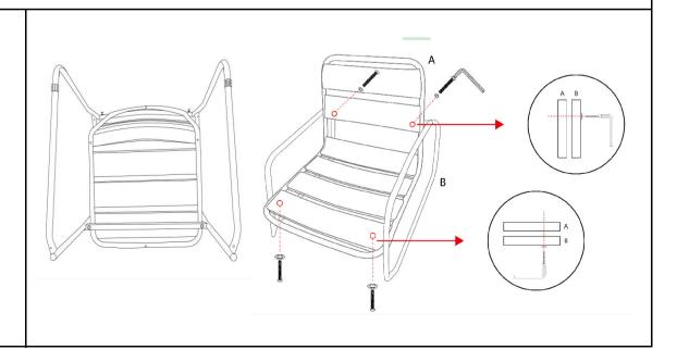
Attach Chair Leg (B) to Chair Seat and Back(A) with Bolts(1) and Washers (2) using the Allen Key (3).
