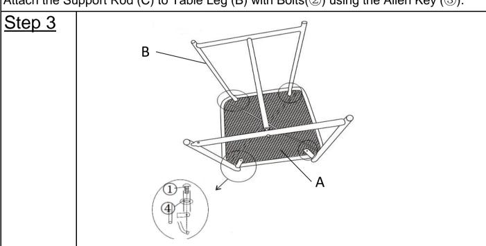
Attach Table Leg (B) to Table Top (A) with Bolts(1) and Washers (4) using the Allen Key (3).
