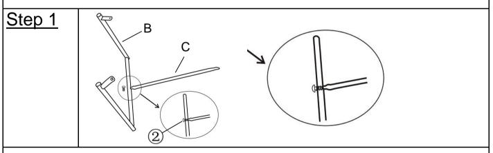
Attach the Support Rod (C) to Table Leg (B) with Bolts(2) using the Allen Key (3).
