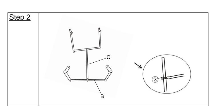
Attach the Support Rod (C) to Table Leg (B) with Bolts(2) using the Allen Key (3).
