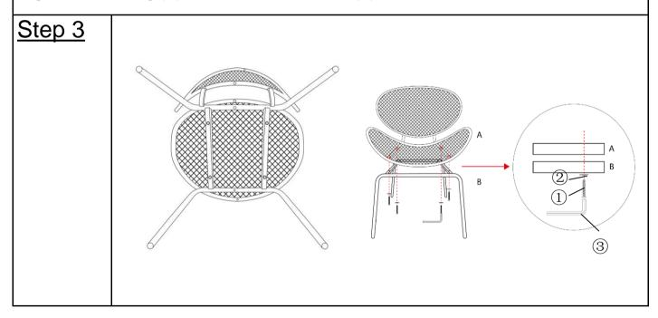
Attach Chair Leg (B) to Chair Seat and Back(A) with Bolts(1) and Washers (2) using the Allen Key (3).
