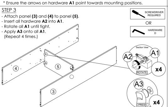
\* In this step hardware A1, A2 and B are pre-inserted.
