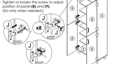
\* In this step hardware J have been assembled in panel (8) and (9).
