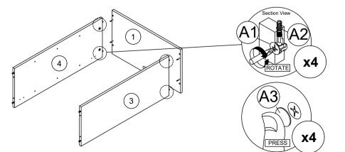
\* In this step hardware A1, A2 and B are pre-inserted.
