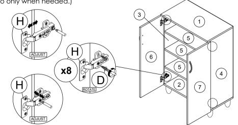
\* In this step hardware H have been assembled in panel (6) and (7).
