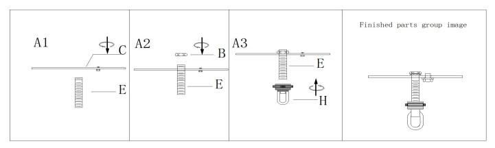
Step A1: Thread the single bar(C) over the nipple (E) a minimum of 6 mm (1/4)". At this point need note that: the side of single bar marked "GND" must face to the down.
