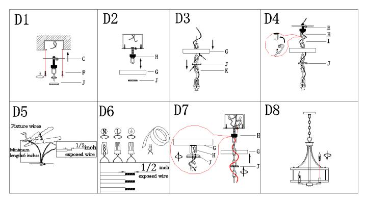
Step D1: Attach the single bar (C) to outlet box with mounting screws (F). The side of single bar marked "GND" must face out, Unscrew the collar ring (J) from the collar loop.
