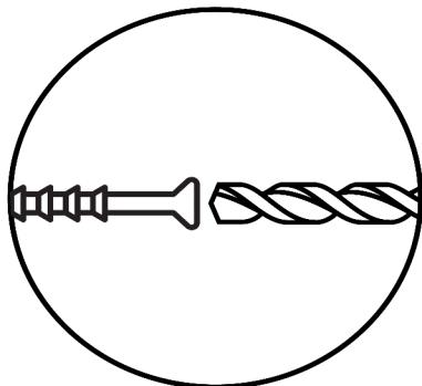
3. Only drill horizontally. Do not force the drill or enlarge the hole for the wall anchor.
