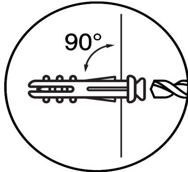
4. Take extra care when drilling into high walls or ceramic tiles. Wall anchors should be a tight fit for the hole. Never use wall anchors in ceilings.
