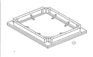
Fix the Leg to the corner of the Apron with Flat Washer, Spring Step 2 Washer and Hexagon Nut, Using the Spanner to tighten it.
