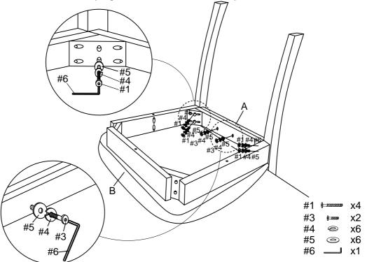
Step 2 . Attach legs (parts C & D) to seat (part B) using bolts (part #2), spring washers (part #4), flat washers (part #5) and allen wrench (part #6).
