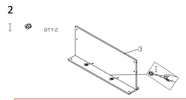
Align back board (#3) to the cam bolts of the middle support, then secure by using cam locks (#I).
