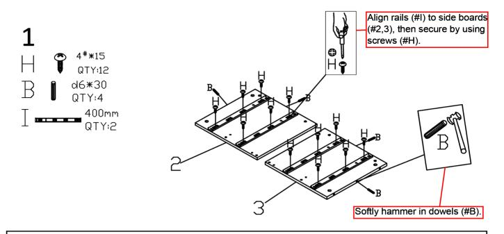
Tip: Place parts on the flat level surface to ease alignment and assemble.
