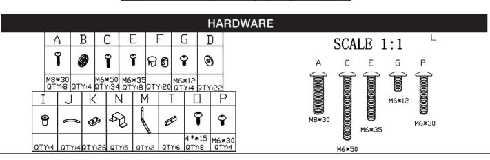
Align side panels (#1,6) to back panel (#3), then secure by using bolts (#C) with washers (#D) to barrel nuts (#F). Once secured, use barrel nut caps (#F) to cover barrel nuts (#F).
