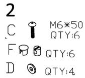
Align middle support (#4) to the product, then secure by using bolts (#C) with washers (#D) to barrel nuts (#F). Once secured, use barrel nut caps (#F) to cover barrel nuts (#F).
