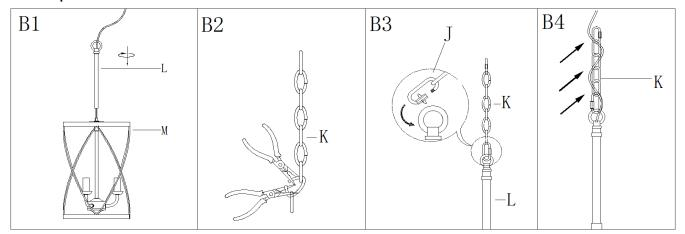
Step B1: Thread the tube (L)onto the fixture body (M) till tight .
