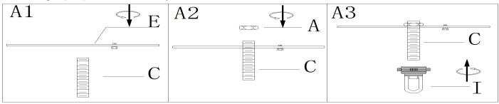
Step A1: Thread the single bar(E) over the threaded nipple (C) a minimum of 6 mm (1/4"). At this point need note that: the side of single bar marked "GND" must face to the down.
