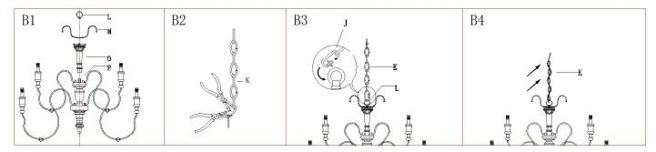
Step B1: Thread the post (O)onto the fixture body (P) till snug; Position the steel holder (L)over the threaded nipple on the top of post (O) till snug, then secure with loop(L).
