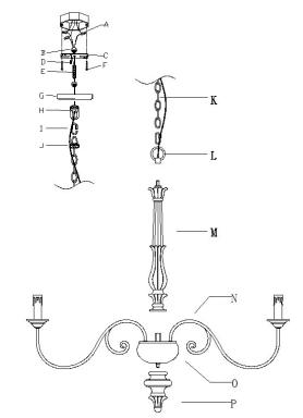
Step A2:Thread the single bar(C) onto nipple (E), thread another hex nut (B)onto the nipple (E), then tighten the nut(B) to secure single bar (C) in place. At this point need note that: the side of single bar marked "GND" must face to the down.
